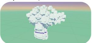
**Grid** - Arranges the objects in a 3D grid. This Replicator Shape ignores the Amount of Replications. Instead the amount of objects created will be dependent on the size of the grid, controlled with **Grid Size**. You can change the how far away the grid layers are on each axis with the **Grid Spacing** parameter.
